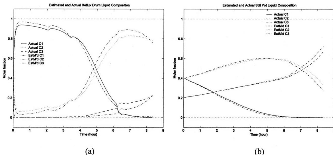
Figure 8. Effect of the period of temperature measurements for  $\Delta t_m = 1$  min. (a) Reflux-drum compositions; (b) reboiler compositions.
