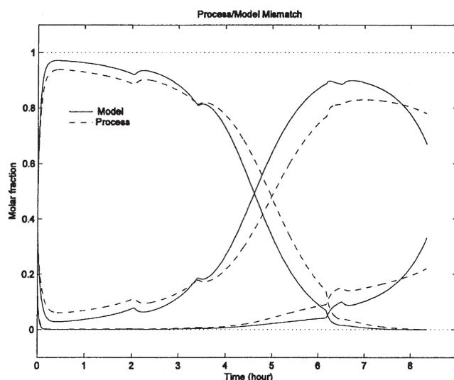
Figure 2. Mismatch between the process and the simplified model used in EKF.
