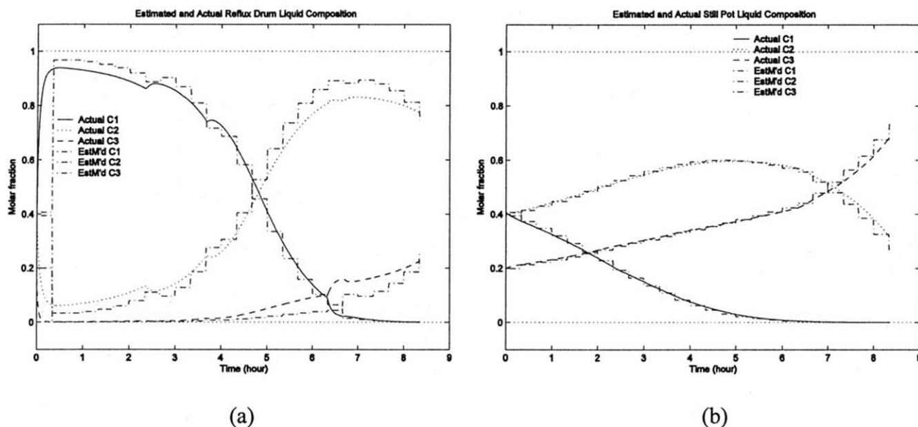
Figure 9. Effect of the period of temperature measurements for  $\Delta t_m = 20$  min. (a) Reflux-drum compositions; (b) reboiler compositions.
