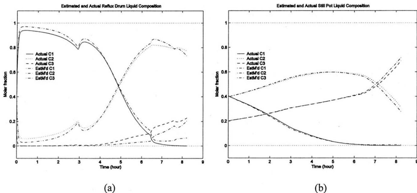
Figure 11. The closed-loop responses of the MBDC under the scheduling controller with actual composition feedback. (a) Reflux-drum compositions; (b) reboiler compositions.
