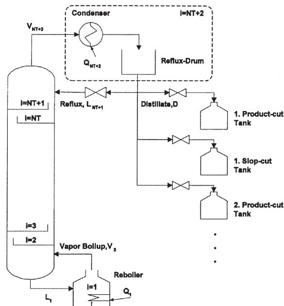
Figure 1. The schematic of a multicomponent batch distillation system.
