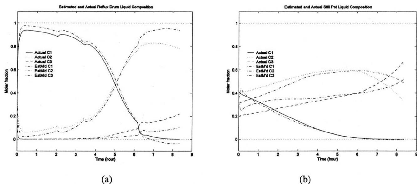
Figure 10. Effect of the initial conditions for  $x_0 = [1/3; 1/3; 1/3]$  and  $P_0 = 0.1$ . (a) Reflux-drum compositions; (b) reboiler compositions.
