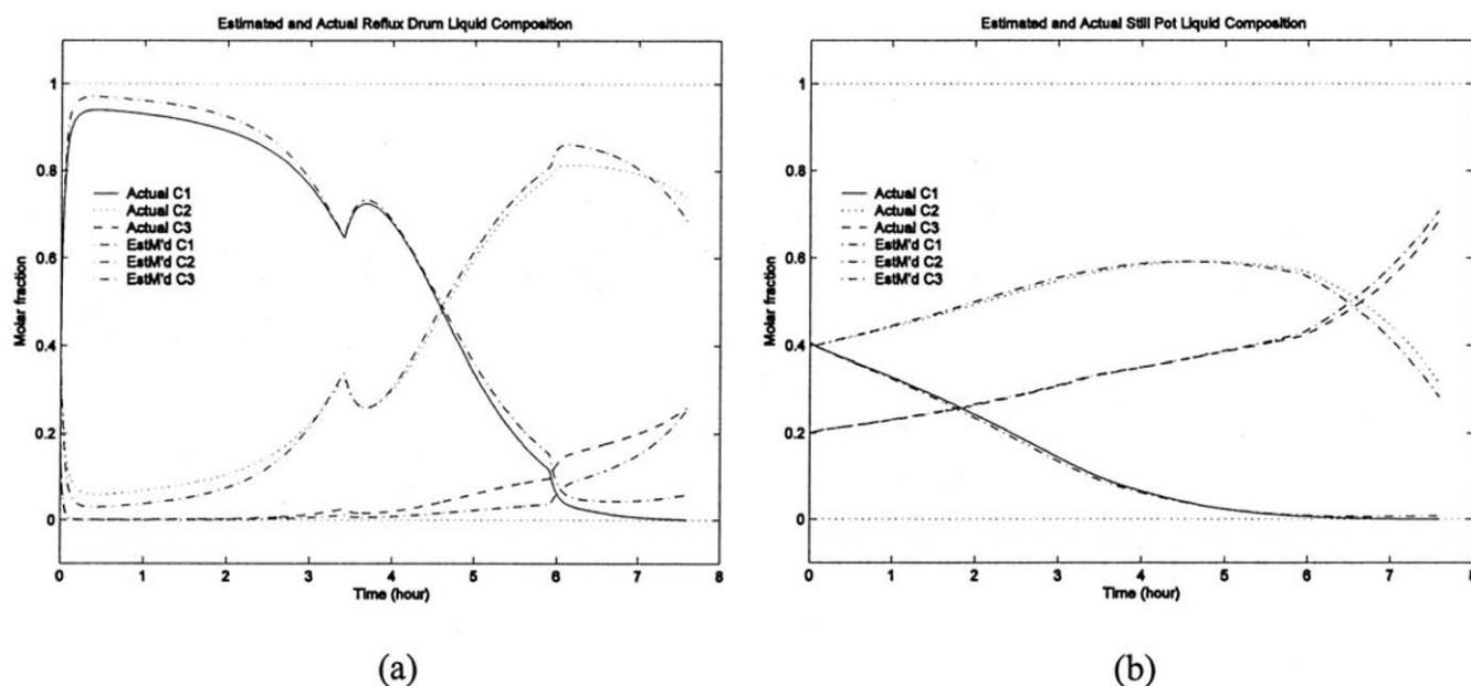
Figure 12. The closed-loop responses of the MBDC under the scheduling controller with estimated composition feedback. (a) Reflux-drum compositions; (b) reboiler compositions.
