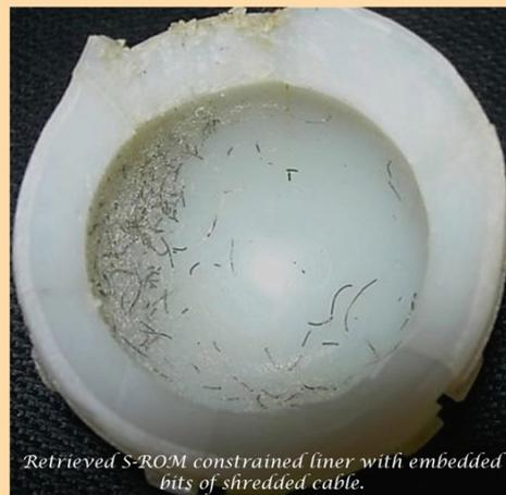
*Retrieved S-ROM constrained liner with embedded bits of shredded cable.*
