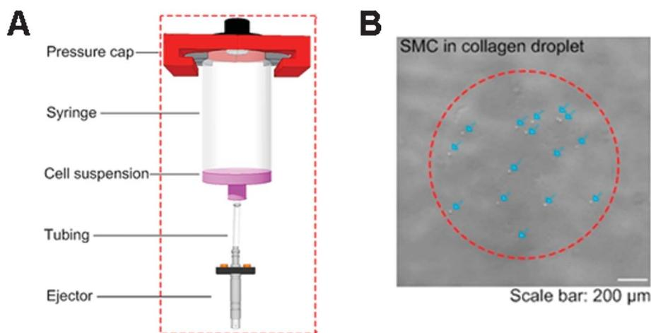
**Fig. 1** (A) Cell encapsulation and microdroplet generation system. (B) A typical printed cell-encapsulating collagen droplet. Arrows represent the smooth muscle cells (SMC) encapsulated in a droplet.
